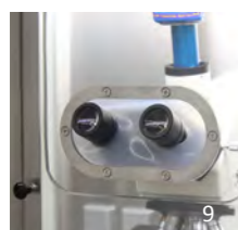
1: Integrated monitor- and weighing worktop; 2: Exhaust air cooler; 3: Integrated RTP-Port; 4: Solutions for compounder; 5: Window in back panel; 6: SC-slucise-isolator corner solution; 7: Training-SC with computer workstation for two people; 8: IV-bar in workspace; 9: Integrated microscope
