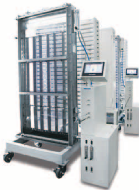
Pilot Scale, Plate Type Photo Bioreactor, Illuminated by External LED Plates
